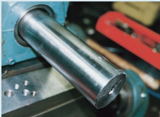
No Fretting corrosion or shaft damage with GRIP TIGHT Adapter Bearing Assembly
